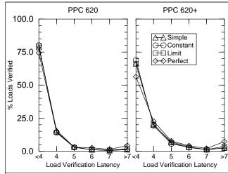
FIGURE 7. Load Verification Latency Distribution. Numbers shown are the percentage of correctly-predicted loads that are verified a given number of cycles after they are dispatched.
