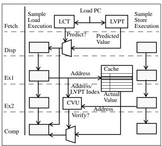
FIGURE 3. Block Diagram of the LVP Mechanism. The Load PC is used to index into the LVPT and LCT to find a value to predict and to determine whether or not a prediction should be made. Constant loads that find a match in the CVU needn't access the cache, while stores cancel all matching CVU entries. When the load completes, the predicted and actual values are compared, the LVPT and LCT are updated, and dependent instructions are reissued if necessary.
